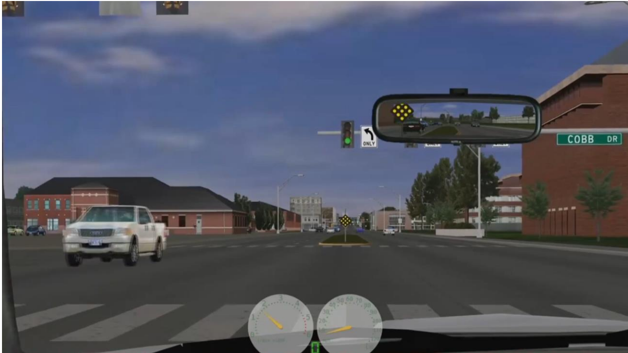
Video demonstration screen capture of the left turn assistance system. This system provides an auditory guidance system for safely navigating intersections. This same system can also provide assistance for other types of intersections.
