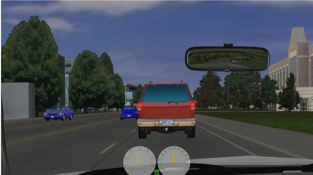
Video demonstration screen capture of the forward collision warning system. The audio alert activates when the vehicle get too close to a vehicle or other object in front of the car based on speed.
